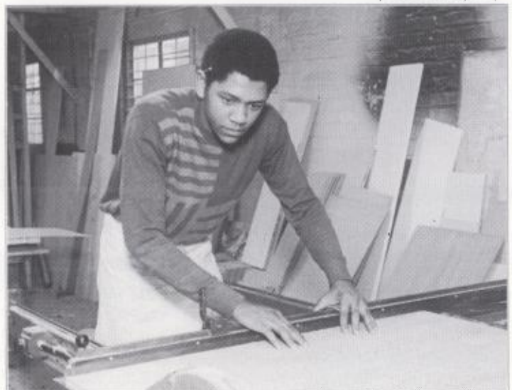
This trainee joiner will be exposed to high levels of formaldehyde-containing dust when the circular saw is used to cut the blockboard
